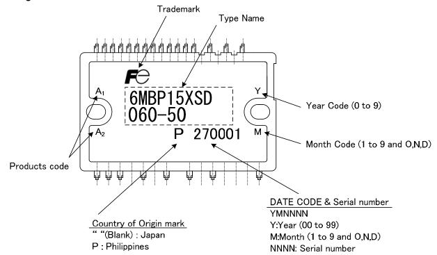
Note : Product code  $A_1$  means current ratings , and "L" is marked. Product code  $A_2$  means variations , and "D" is marked.
